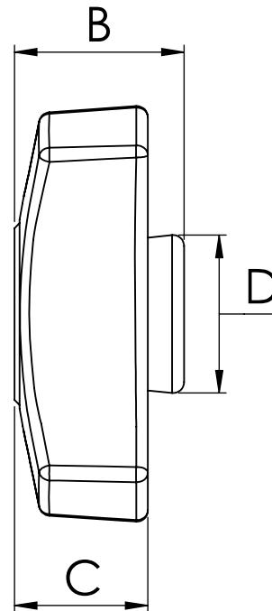
NOTE: M6 x 1.0 aluminum insert has 6.5mm length of thread.
